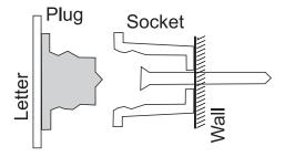
Then press the plug with the letter into the spacer sleeve, until it snaps into place.
